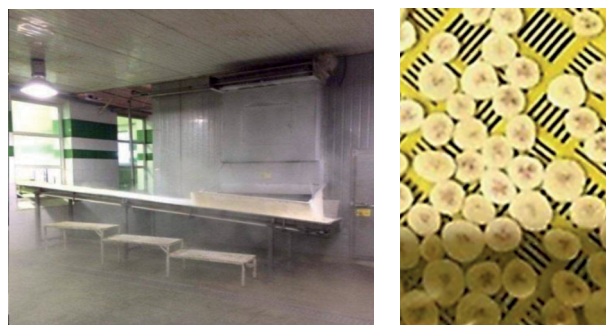
Figure 2. IQF tunnel freezer (left) and the frozen banana slices (right)
